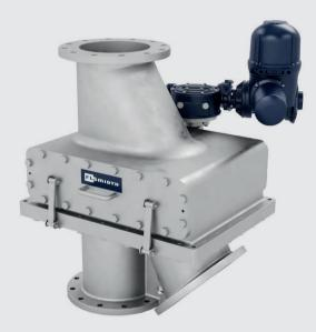
The SK V2 two-way valve is available in five sizes: 150mm (6"), 200mm (8"), 250mm (10"), 300mm (12") and 350mm (14") and matches the I.d. of standard schedule 30 pipe. Flanges are available in ANSI or DIN designs, with 45° divert port as standard.
